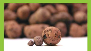
EXPANDED CLAY AGGREGATE (ECA)
