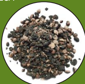
2 - 8 mm crushed ECON ( Expanded Clay Aggregate for Construction ) Structural Concrete Applications
